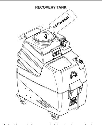
Add a defoamer in the recovery tank to reduce foam, prolonging the life of the Spyder  $^{\text{TM}}$  vacuum motor .
