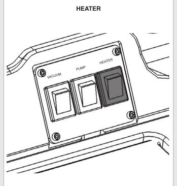
Release tool trigger. Turn on heater. Wait 8-10 minutes for unit to pre-heat. Once heated, re-key upholstery tool until hot water begins flowing. Once hot water is flowing, release trigger and pre-heat an additional 4-5 minutes.
