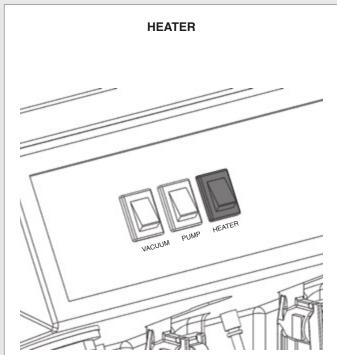
Release tool trigger. Turn on heater. Wait 8-10 minutes for unit to pre-heat. Once heated, squeeze cleaning tool trigger again until hot water begins flowing. Once hot water is flowing, release trigger and pre-heat an additional 4-5 minutes.
