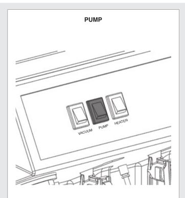
After the machine has been plugged into a 20 amp grounded outlet. Turn on pump. Squeeze cleaning tool trigger until it releases a steady flow.
